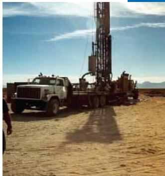
Drilling bore holes for sampling of water table
